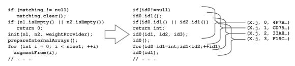
Figure 7.6: The original file named X.j (left), its normalization (center), and the corresponding clone index (right).
