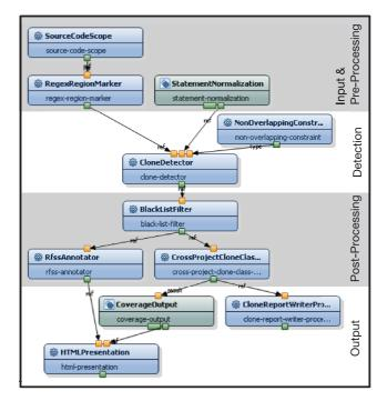
Figure 7.2: Clone detection configuration
