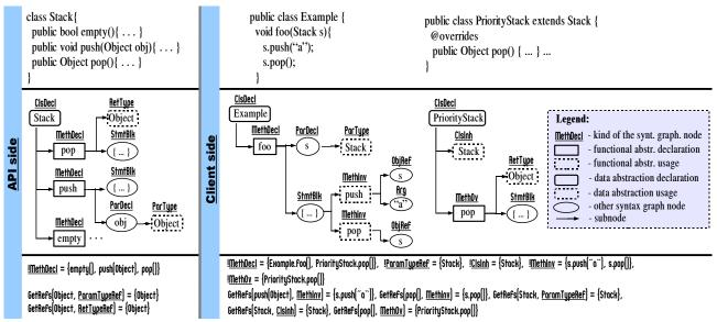
Figure 3. Defining and using stacks
